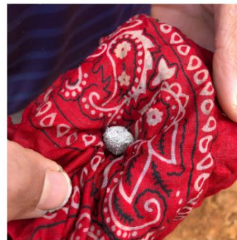
Amalgam after washing mats in buckets and gathering concentrate and mercury added or recovered from pits
