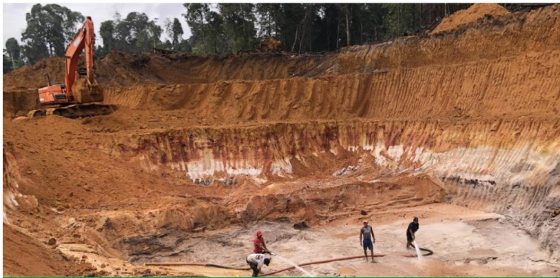
1) Excavator clears vegetation, opens pit and piles material for processing 2) 4-8" suction pumps with 2-4" spurting hoses (jets) create slurry from open pit face or piled material
