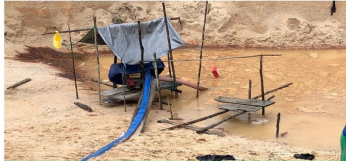
2-4" suction pumps used by pump men to work tailings/ mined out pits. Pit edge typically washed using a spurting hose.
