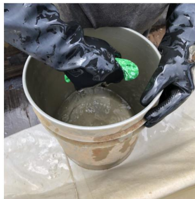
7) The mercury-gold amalgam is collected in a cloth
