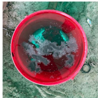
Amalgam after washing mats in buckets and gathering concentrate and mercury added or recovered from pits
