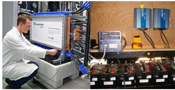
25 kW redox battery developed by Fraunhofer (left) and a simple car-battery based system developed by Omega Telecom in Trinidad & Tobago for an off-grid solar energy supply system (right)
