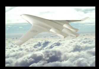
Hugo Junkers' 1924 design for a giant flying wing. The wing was to accommodate 26 cabins for 100 passengers, carry a crew of 10, and have enough fuel for 10 hours of flight. http://www.century-of-flight.net/Aviation%20history/flying%20wings/Early%20Flying%20Wings.htm
