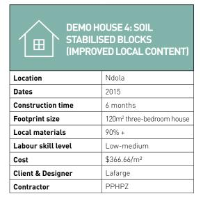
A three-bedroom house using SSBs. An evolution of Demo house 3, Demo house 4 uses locally produced concrete tiles on the roof, and timber framed windows and doors crafted by local MSMEs. Thus the house features almost 100% local content.
