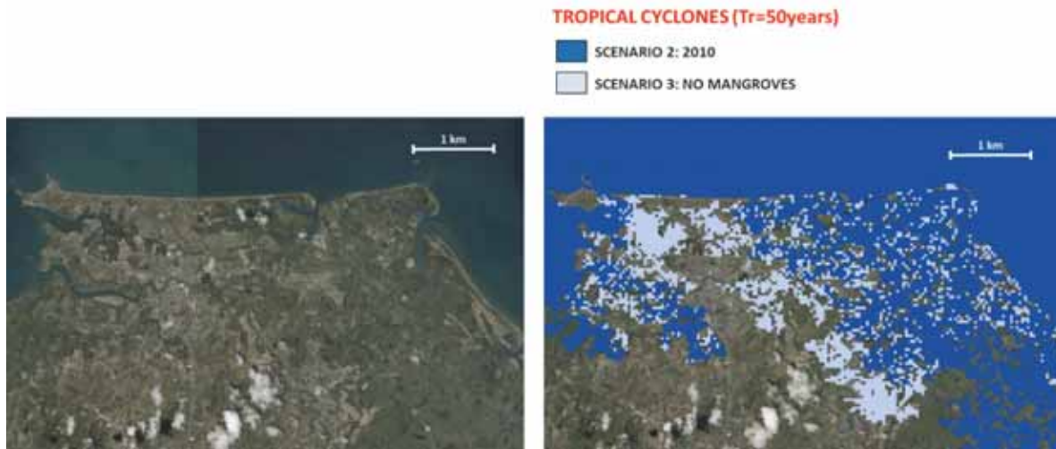
Figure 35 Flooding mask in Roxas for 50 years return period event in the Tropical Cyclones data. The light and the dark blue polygons in the figure on the right represent water and flooding of land under the two different scenarios.
