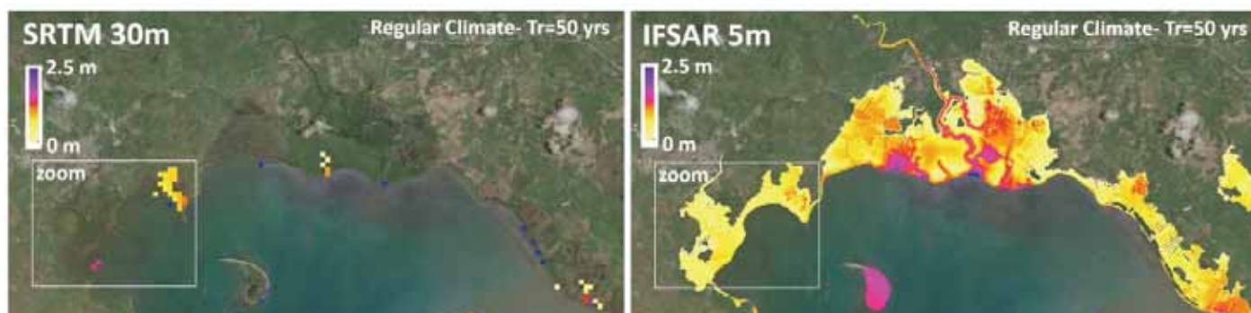
Figure 40 Flood Height in Pagbilao for 50 year return period event under regular conditions with current mangrove cover. The left image shows the SRTM 30m, the right image shows IFSAR 5m.
