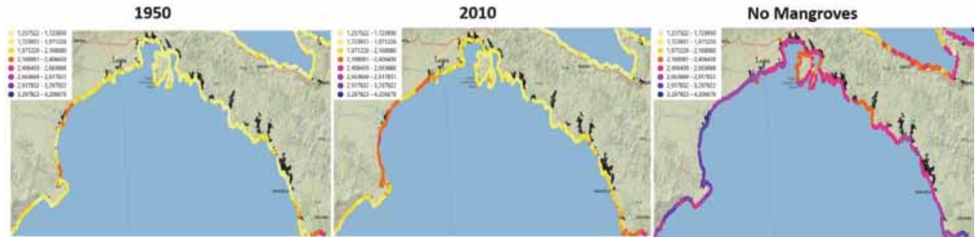
Figure 30 Flood height in Pagbilao for 50 year return period event under tropical cyclone conditions for the three scenarios of historical, current and no mangroves. The values are water or flood height at the coast ranging from -1m (yellow) up to -5m (blue).
