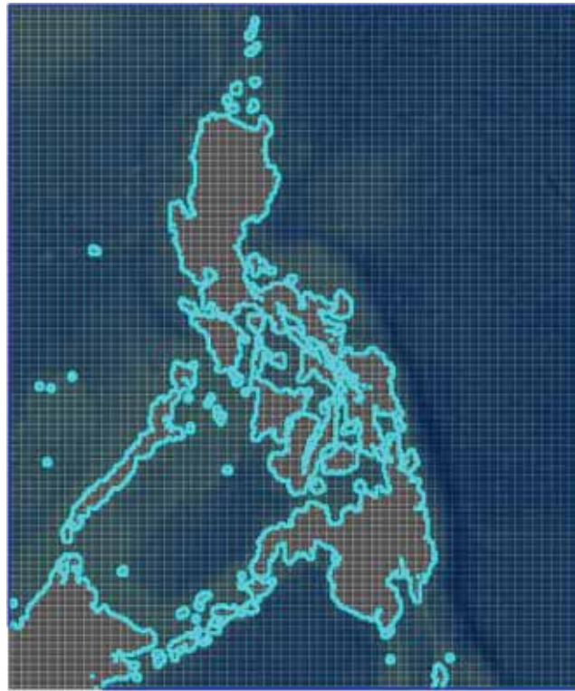
Figure 6.2 The 5 Km grid used for the baseline storm surge study, coastal points where waves and sea levels are obtained are highlighted in cyan.
