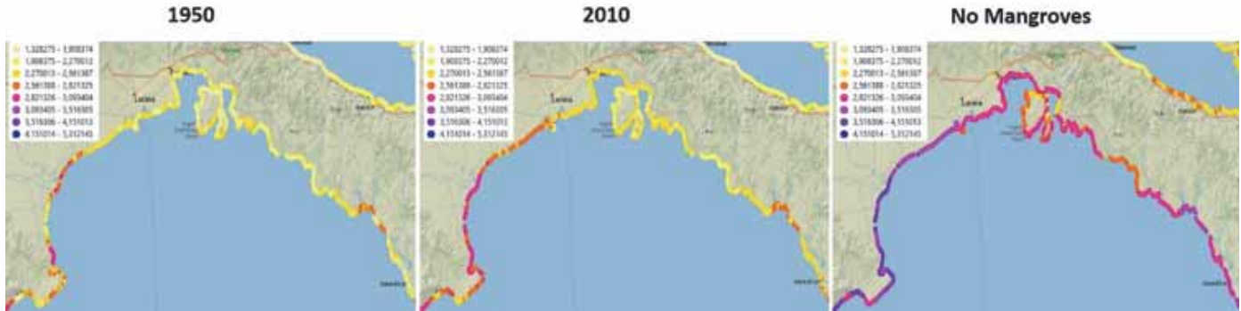
Figure 29 Flood height in Pagbilao for 25 year return period event under tropical cyclone conditions for the three scenarios of historical, current and no mangroves. The values are water or flood height at the coast ranging from -1m (yellow) up to -5m (blue).
