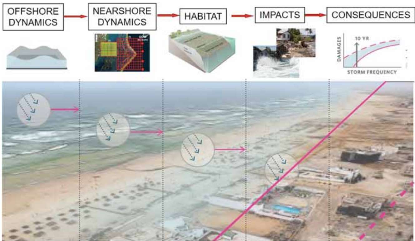
Figure 3 Methodology to evaluate coastal protection services of ecosystems like coral reefs and mangroves. 1: Oceanographic data are combined to assess offshore sea states. Stage 2: Waves are modified by nearshore hydrodynamics. Stage 3: Effects of habitat on wave run-up and surge are estimated. Stage 4: Flood heights are extended inland along profiles (every 200 m) for four locally generated, storm events (10, 25, 50, 100-yr events) with and without mangroves. Stage 5: The land, people and built stock damaged under the flooded areas are estimated (see World Bank 2016).
