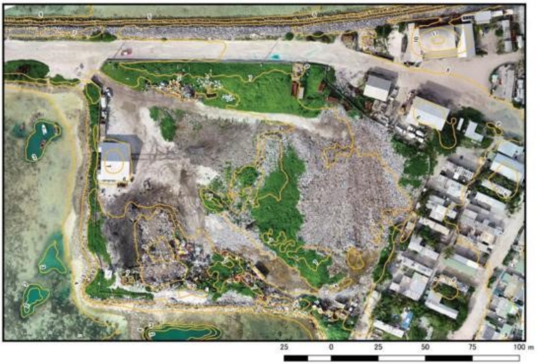
Figure 12: Aerial image of the disposal site taken by drone (with contours above sea level), June 2018 (Source: KASWMP)
