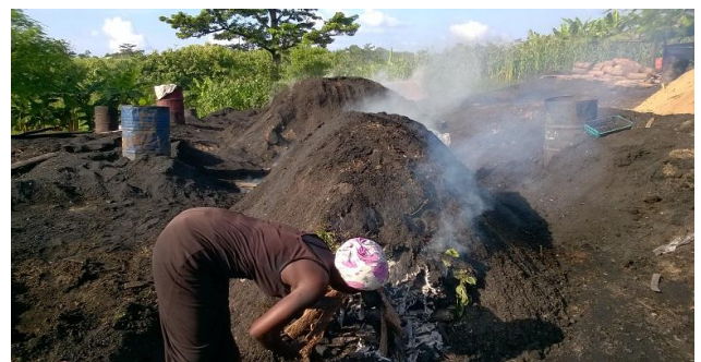
Picture 10: Earth mound Pit kiln for charcoal making
