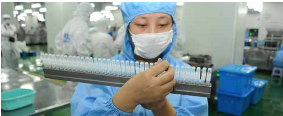
VISUAL INSPECTION OF CLEANLINESS OF MEDICAL DEVICE AFTER CLEANING USING NON-ODS SOLVENT. PHOTO CREDIT: FECO/MEP, CHINA
