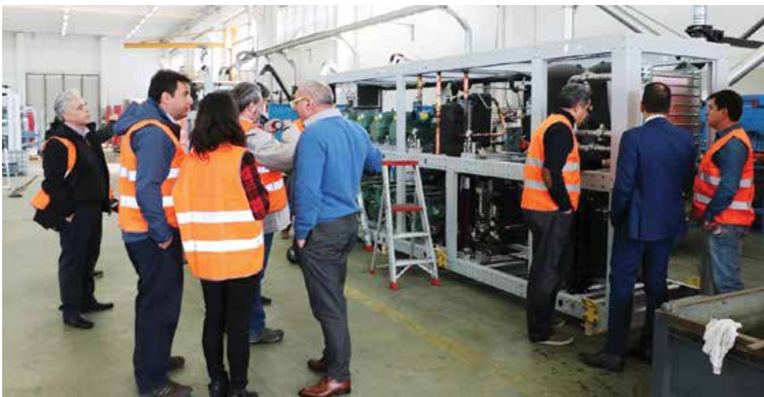
TRAINING OF TECHNICIANS IN CHILE ON TRANSCRITICAL CO 2 TECHNOLOGY. PHOTO CREDIT: NATIONAL OZONE UNIT, CHILE
