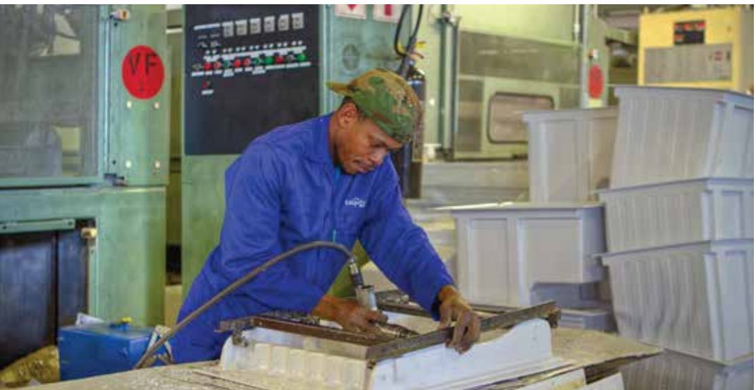
FINISHING WORK ON FRIDGE DOOR PANELS FORMED USING CYCLOPENTANE AS BLOWING AGENT AT PALFRIDGE. PHOTO CREDIT: PALFRIDGE
