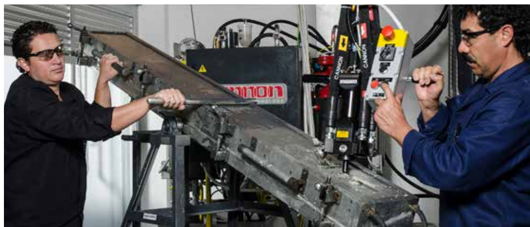
FOAM PANEL TESTING AT ESPUMLATEX USING A BRETT MOLD. PHOTO CREDIT: ESTEBAN GARCÍA, ESPUMLATEX
