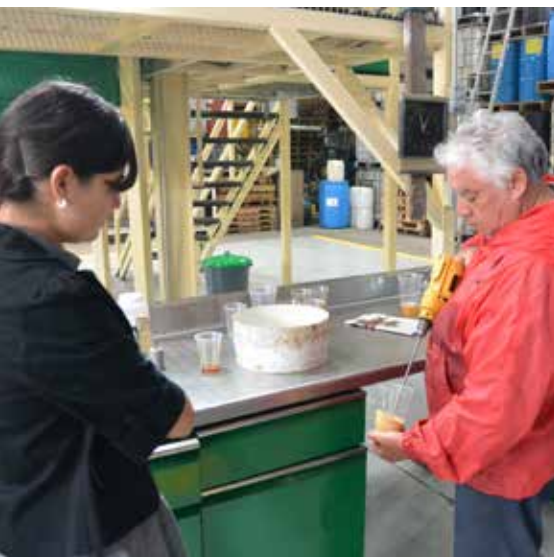
HAND TESTING PU FOAM SYSTEM AT COMSISA SYSTEM HOUSE IN MEXICO. PHOTO CREDIT: HORACIO HERNÁNDEZ DEL CASTILLO
