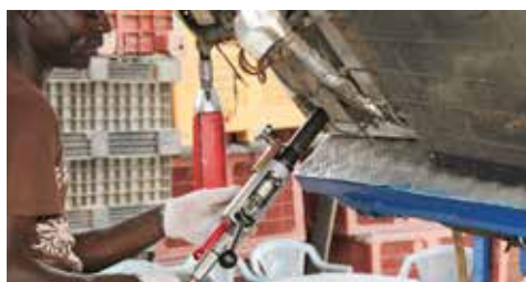
EMPLOYEE AT CITY WASTE MANAGEMENT COMPANY LIMITED PROPERLY DEGASIFIES A REFRIGERATOR BEFORE ITS DISMANTLING. PHOTO CREDIT: THE PROJECT TEAM
