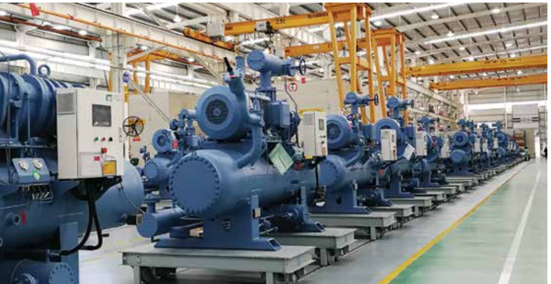
COMPRESSOR UNIT ASSEMBLY LINE AT FUJIAN SNOWMAN CO. LTD., CHINA. PHOTO CREDIT: FUJIAN SNOWMAN CO. LTD
