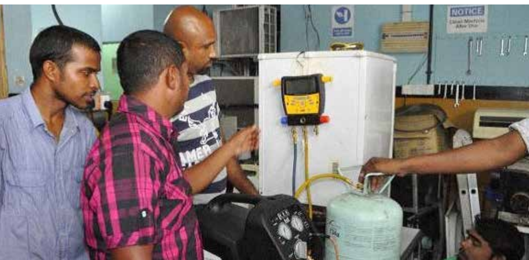
RECOVERY OF REFRIGERANT USED IN THE FISHERY SECTOR. PHOTO CREDIT: MIT AND NATIONAL OZONE UNIT, MALDIVES
