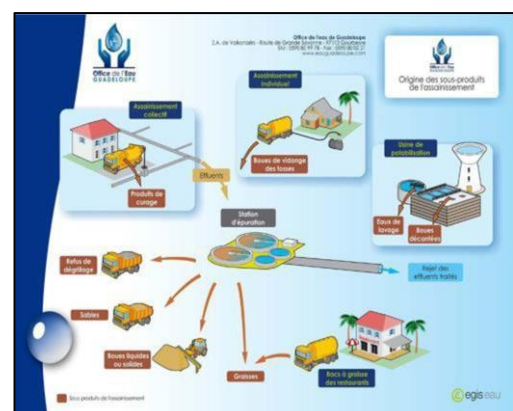
Figure 10: Urban Water Treatment Processes (excluding by-product reuse)
