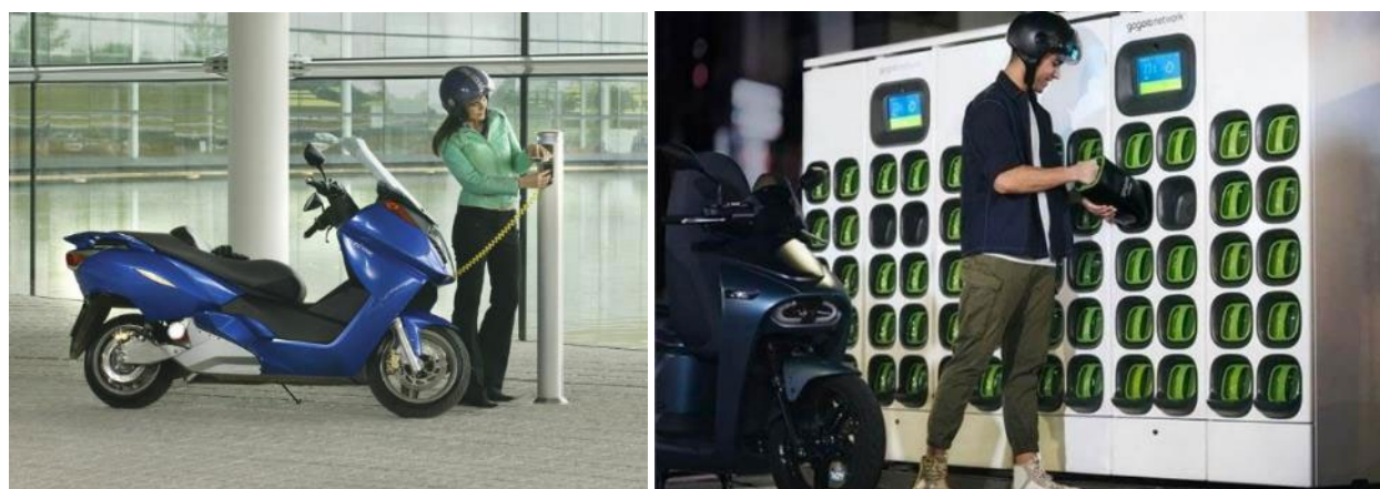
Figure 31. Plug-in Charging System (Left) and Battery Swapping System. Search Engine (2023)
