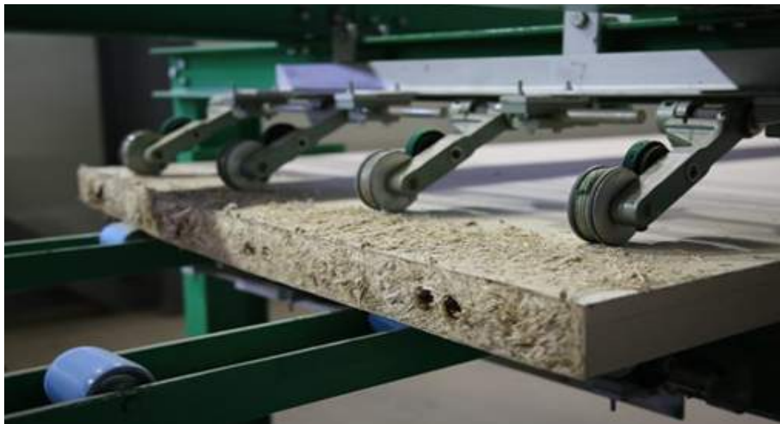
Figure 31: Manufacturing process for straw panels
