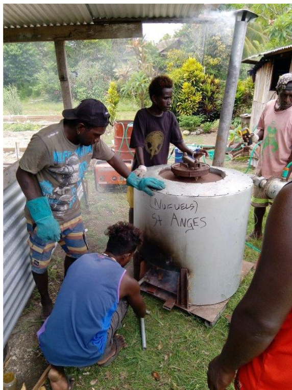
Figure 5 Community scale pyrolysis unit (Solomon Islands) 34
