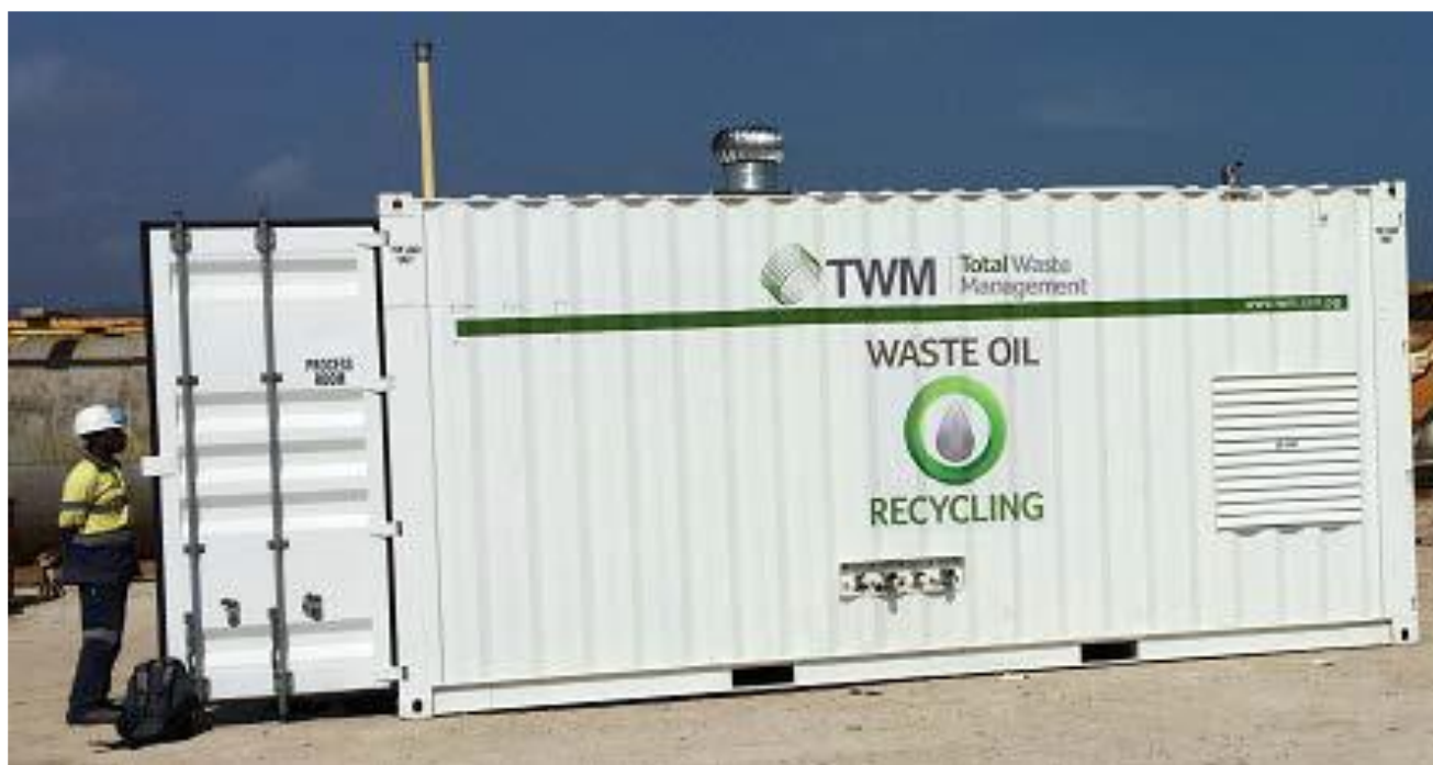
Figure 8 Containerised used oil processing and fuel blending unit (PNG) 35
