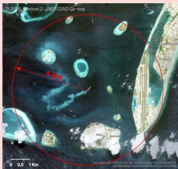
Figure 5: Satellite-derived sediment plume in Northern Malé Atoll (Maldives) on 29 July 2020, illustrating the dispersion of suspended sediments associated with marine sand dredging activities
