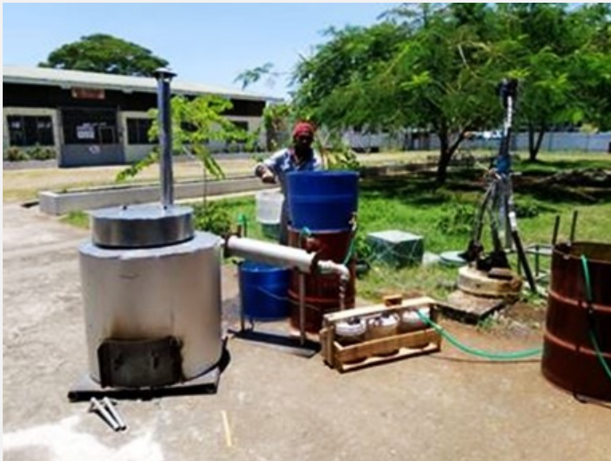
Nufuels Limited small-scale pyrolysis system in the Solomon Islands Image Source: WasteMINZ, 2011
