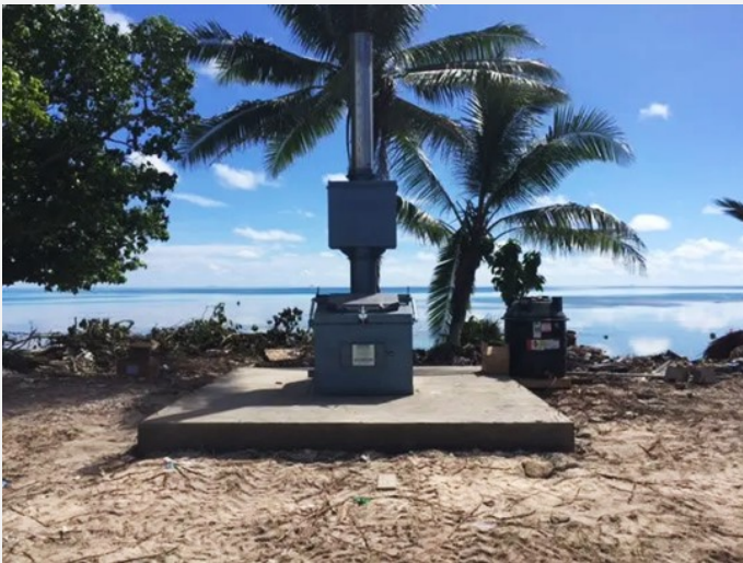
Inciner8 combustion reactor in Kiribati, Tonga, Tuvalu, and Vanuatu for medical waste (note this is combustion only, without energy generation) Image Source: Inciner8, 2016
