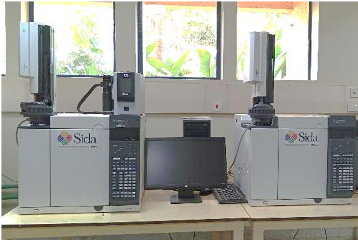
❖ Gas chromatography (GC-FID and GC-ECD with thermal desorption )
